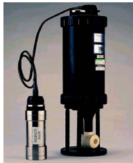
Oceanographic package showing Conductivity – Temperature probe
